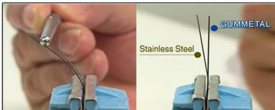
Fig. 1: GUMMETAL® facilitates stable wire bending while offering excellent springback properties
