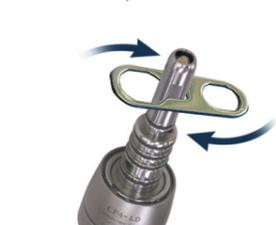
Screw the cover back on with your fingers and then tighten it up with the square hole in the cap tool.
