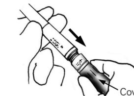
Hold the cover nut, and slide the handpiece straight onto the coupling until it clicks securely into place.
