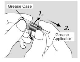
(1) Rotate the grease applicator to apply grease (lubricating oil) to the end of the grease applicator.
