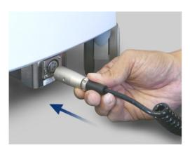
Plug the cord for the foot switch into its mate on the Main unit. Make sure it clicks securely into place.
