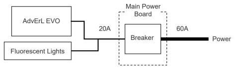
Example of circuit that is not likely to cause fluorescent lights to flicker. Use separate breakers for this device and fluorescent lights.
