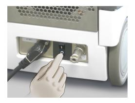
(5) Turn off the circuit protector at the bottom of the back of the Main unit.
