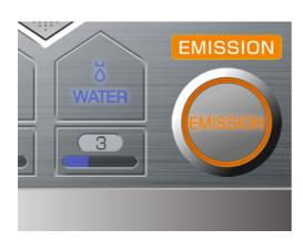
(4) Depress the foot switch all the way down to emit the laser. The Ready Key will change to Emission, and the device will make a continuous beeping sound.
