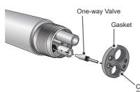
Take off the gasket with a needle. Take out the oneway valve. Slide a new valve into place. Put the gasket back on in its original position.
