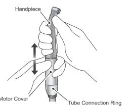
Hold the motor cover and pull the handpiece straight off
