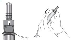
Apply a small amount of the LS OIL or MORITA MULTI SPRAY to the O-ring, and then slide the motor cover straight onto the micromotor. Plug it in until there is an audible click.
