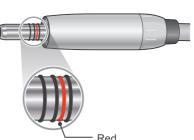
Remove the O-rings with tweezers or another such tool and install the replacements. Make sure that the red O-ring is in the right place.
