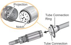
Line up the projection on the micromotor connection with the notch in the tube connection and slide the tube onto the micromotor. Then tighten up the tube ring securely.
