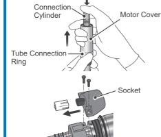
Holding the tube connection ring, grip the motor cover and press down on the connection cylinder with your thumb to slide the cover off the micro-
