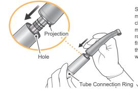
Slide the handpiece straight onto the micromotor's connection cylinder until it clicks securely into place. For handpiece models equipped with a light, slightly rotate the handpiece so that its projection fits in with the hole on the micromotor. If the projection and hole fit properly, there will be a clicking sound.
