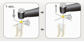
Press down for approximately 1 second to prevent the file backing out then pull it up. Repeat the sequence until the meter reaches the position 0.5 as shown in the illustration on the right. When the meter reaches 0.5, the file rotation stops automatically.
