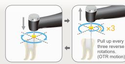
Advance the file slowly to start canal shaping. When the file starts rotating in the reverse direction, pull the file up quickly; repeat the sequence. When the meter reaches the set point 1, the file rotation stops automatically.
