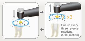
Advance the file slowly to start canal shaping. When the file starts rotating in the reverse direction, pull the file up quickly; repeat the sequence. When the meter reaches the set point 1, the file rotation stops automatically.
