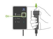
The exposure will begin in a few seconds. The cephalo slit will start moving. The Emission LED (yellow) on the control box will light up and the melody will sound.
