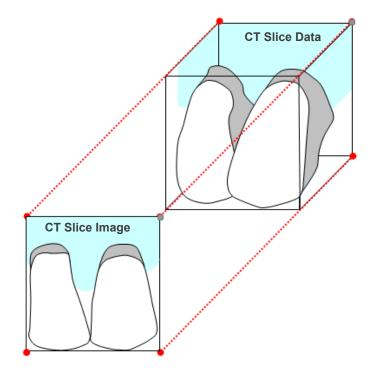
When measuring the target on a CT slice image which has been distorted by the thickness of the slice, the measurement error is only in the vertical direction.
