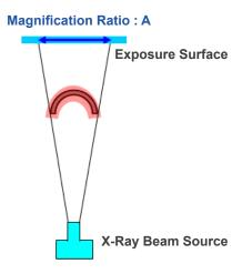
If the image layer is not positioned as shown in the diagram above, the magnification ratio of the image will be larger or smaller.
