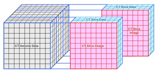
The thickness of the slices creates some distortion in the three dimensional quality of the CT slice data, and this is reflected in the slice image.
