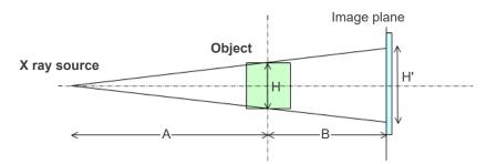
In case of distance measurement on the screen, the distance is measured at the position of object.
