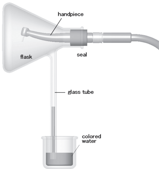
Fig. 1 Complete test setup: Measuring suck-back pressure of the whole handpiece head.
